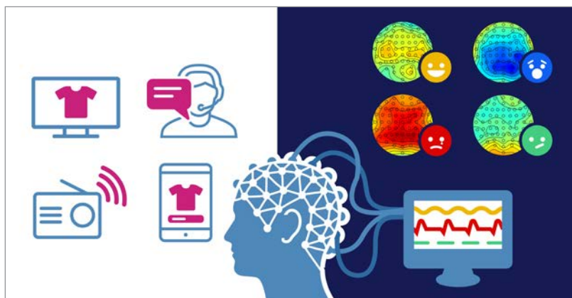
Measuring emotional impact with EEG by comparing with previously classified emotions, classification achieved with machine learning technology.
